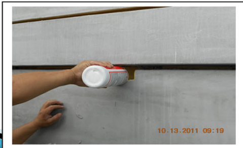
3 4 th floor water poured behind EPS
